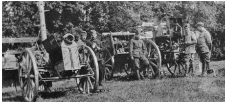
Telefunken D Type 14 was a German heavy field radio station designed in 1914, shown with Polish crew (1920). Transported in 3 limbers/carts. Transmitter: quenched spark gap, power 1.5 kW, frequency 142-500 kHz. Receiver: 2-circuit detector type E85c (43/137-2000 kHz). Aerial: umbrella type with 30 m telescopic mast.
