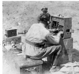
ROD Receiver (Radiostacja Odbiorcza Dywizjonu) was comprised of a French A1 receiver and amplifier type 3ter fitted in wooden suitcase. The Amplifier type 3ter had 3 type TM or R valves, one could function as detector. 2 headphones could be connected. Power source: 90 V HT dry battery and a 4 V accumulator. Weight of complete set was 100 kg. It could be transported by 3 men. Range: 40 km.
